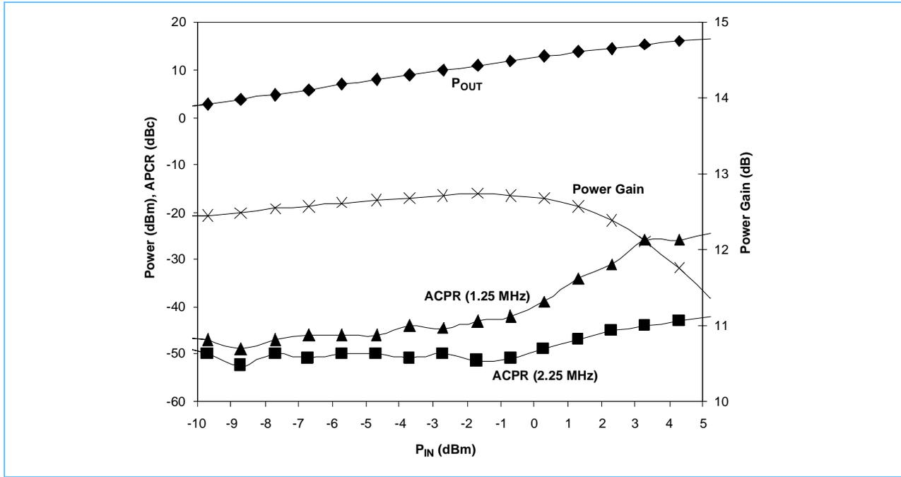
**Measured Performance of SiGe Prototype Driver Amplifier** (See Prototype Test Circuit on page 3.  $T_A = +25^\circ\text{C}$ , Freq.=1900MHz,  $I_{CQ} \approx 5.4\text{mA}$ ,  $V_{BE} \approx +0.823\text{V}$ )
