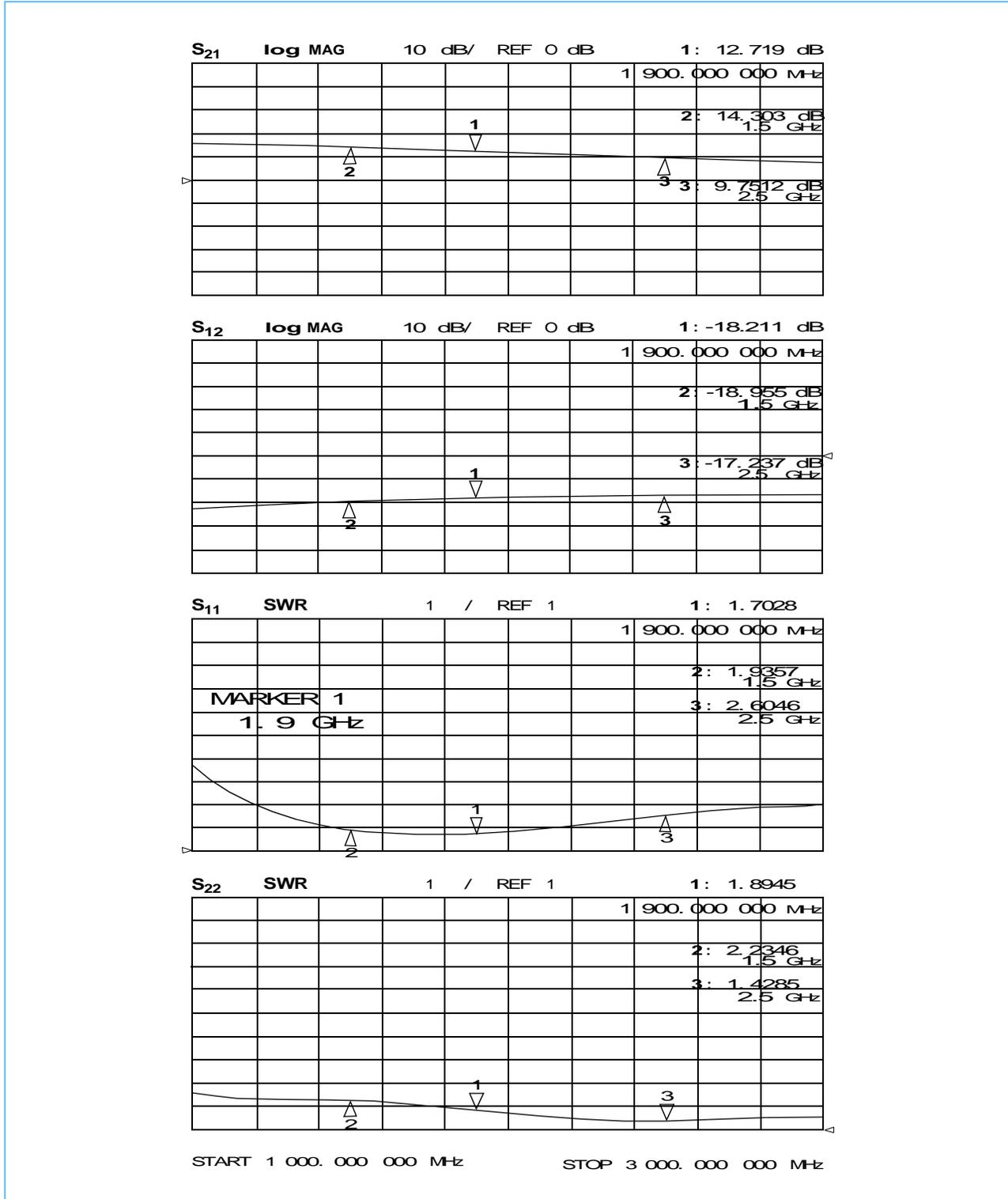
**Measured Performance for Prototype CDMA High Input IIP3 Low Noise and Driver Amplifier Test Circuits** (See Prototype Test Circuit on page 3.  $T_A = +25^\circ\text{C}$ , Freq.=1900MHz,  $I_{CQ} \approx 5.4\text{mA}$ ,  $V_{BE} \approx +0.823\text{V}$ )
