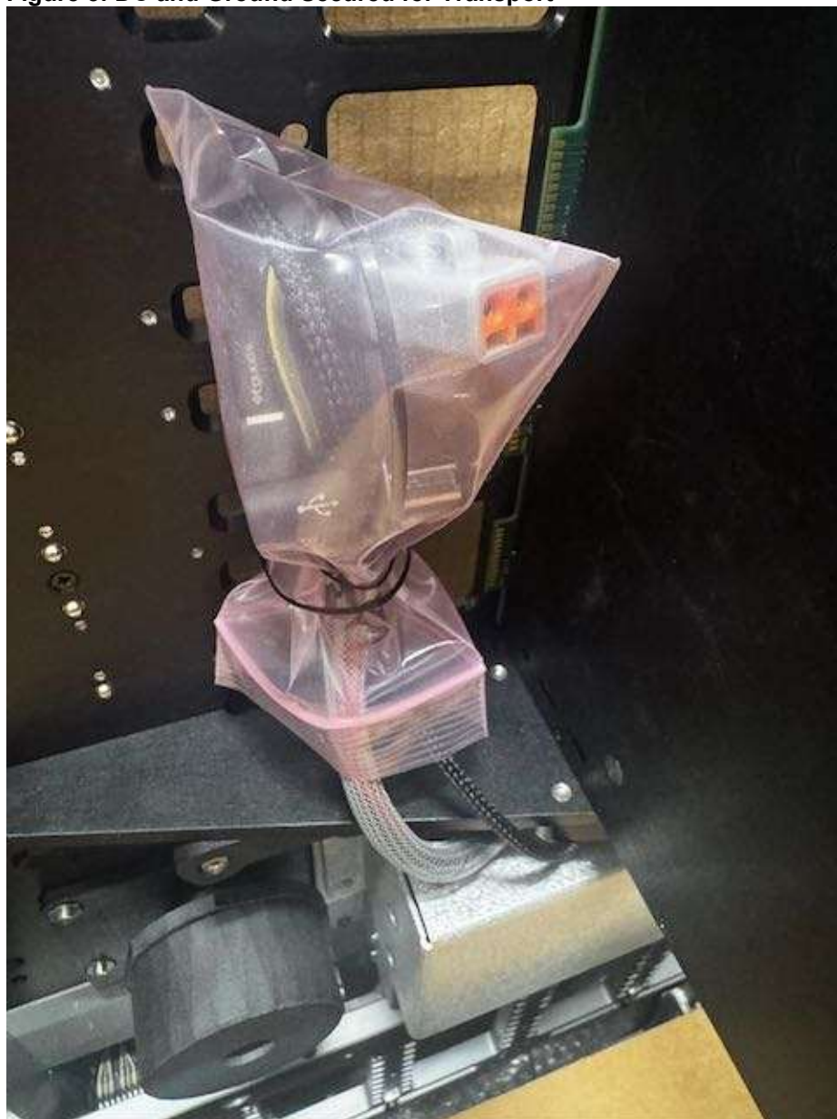
Figure 5: DC and Ground Secured for Transport
