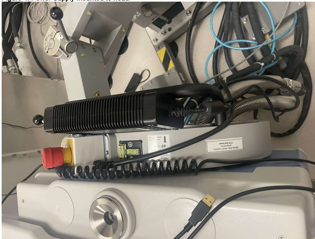
Figure 4: Power Supply mounted to head
