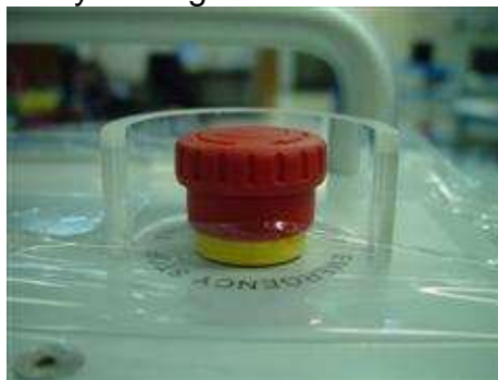
Cassini 16 - Emergency Power Off (EPO)
