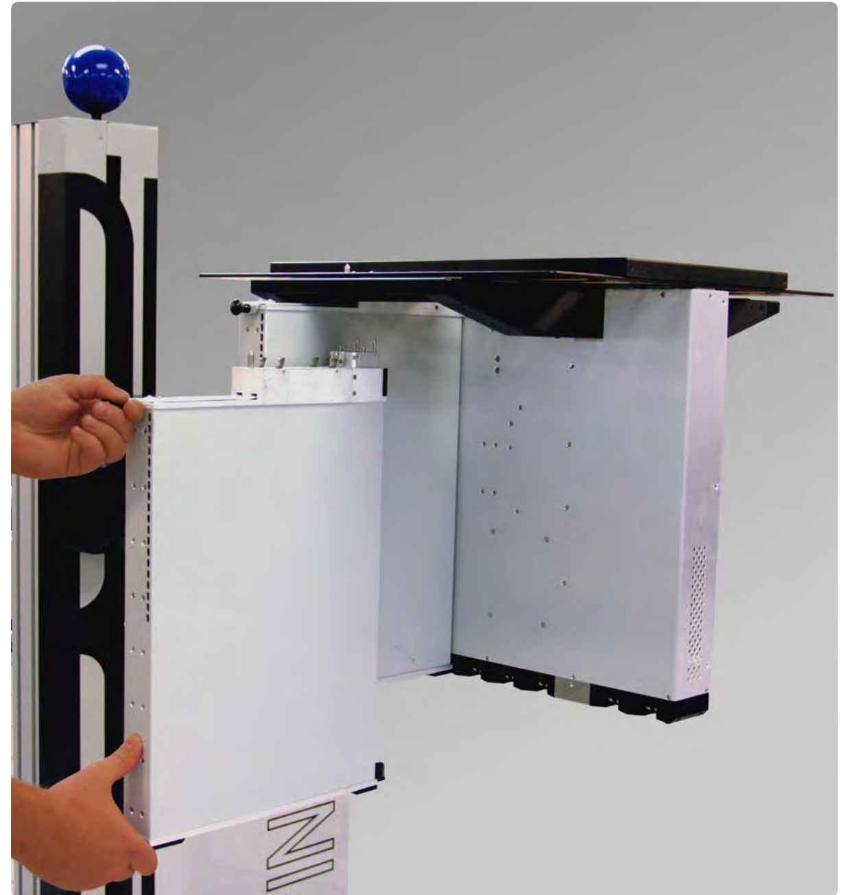
FIGURE 1.38 REMOVING TIMS FROM THE TEST HEAD
