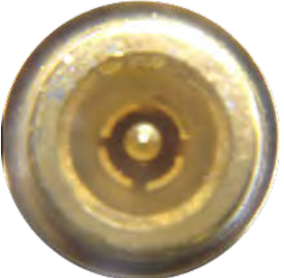
FIGURE 3.6 CLEAN PKZ #12 CONNECTOR EXAMPLE
