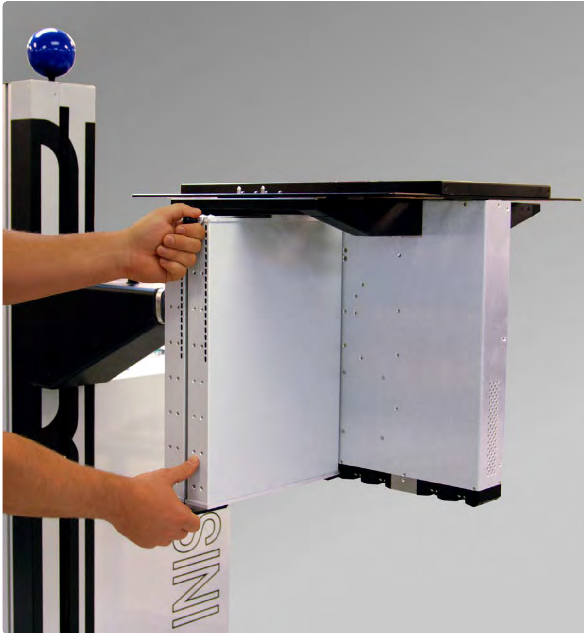
FIGURE 1.37 ADDING TIMS TO THE TEST HEAD
