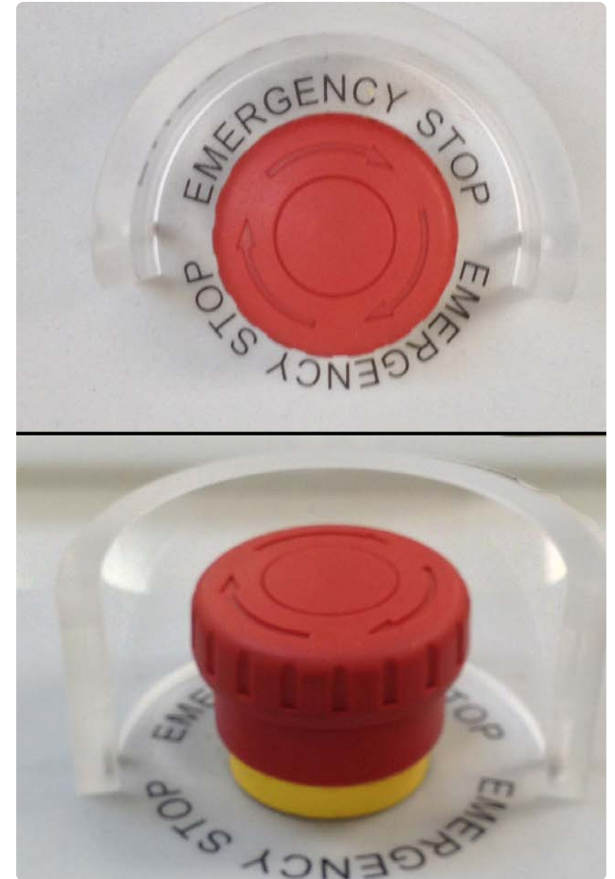
FIGURE 1.4 EMERGENCY OFF (EMO) SWITCH
