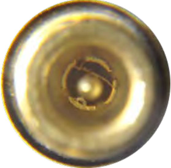
FIGURE 3.5 DIRTY PKZ #12 CONNECTOR EXAMPLE
