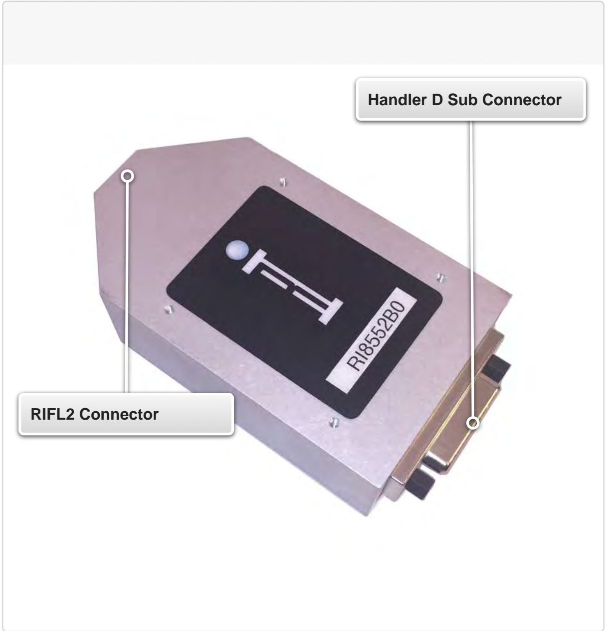
FIGURE 1.52 GPIB HANDLER OR PROBER POD (RI8552B)
