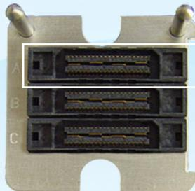
**Digital Block:** 40-pin, high-speed connector
